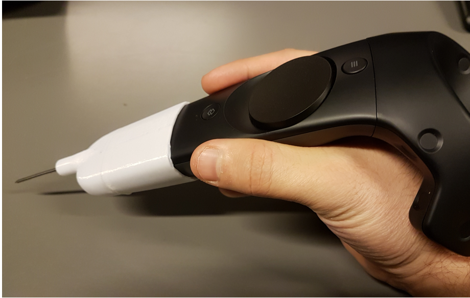
Fig. 1. The needle used for the experiment, made from a 3D printed mount and a nail attached with a bolt in the loop designed for the wrist strap.
