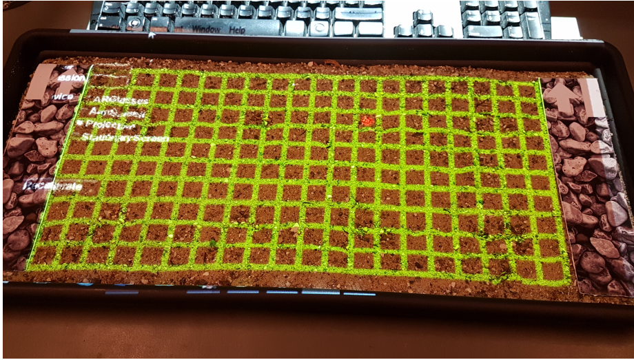
Fig. 5. The grid projected onto the sand with the targets shown as a red dot. [5]
