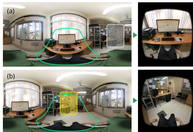
Fig. 3. a) Equirectangular frame with an active hotspot (grey region), the region of user's POV (within green outline) and corresponding user's view (right) in Schrödinger's Vada-Pav . b) Hotspot detected (yellow region) within the POV and corresponding user's view (right)
