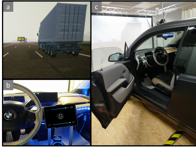
Fig. 2. Three images showing the simulator study setup: (A) The projected driving scenario during an overtake. The distance to the followed vehicle is shown in yellow (B) The dashboard of the car showing the ambient lighting LEDs around the wheel and along the passenger side. On the right, the tablet is shown depicting the continuous ASAM scale. (C) The driving simulator showing the stationary car and the projected driving scenario.
