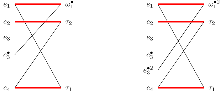
Figure 26: An example with c_f^- > c_f : another variation on the clutch. The previous mode determines \omega_2^{\bullet 2} , hence \omega_2^\bullet is no longer a dependent variable when entering the new mode. Maximal cardinality matchings for N = 1 (left) and N = 2 (right) are shown. Subsequently applying the Dulmage-Mendelsohn decomposition on the left-hand graph returns \beta_\Sigma = \mathcal{G}_F , hence Line 6 of Algorithm 10 returns H = \emptyset . No equation of the new mode is satisfied at the first instant and we move to the next instant. The same holds for the right-hand graph.
