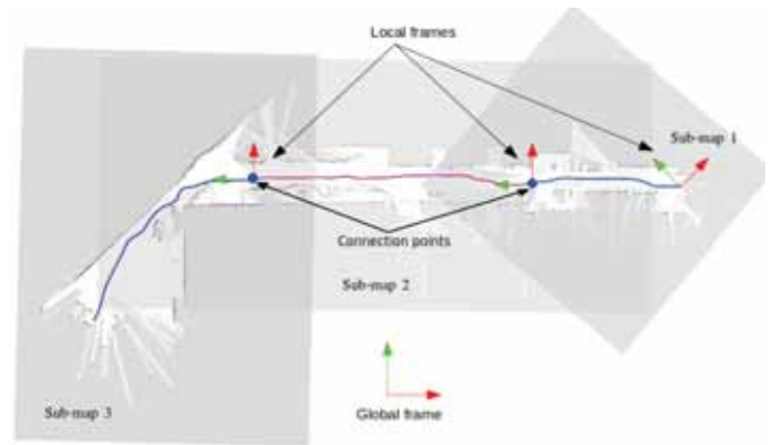
Fig. 1. We represent the vehicle's path (from right to left) in a chain of sub-maps. Each submap is connected to the previous and the next one through connection points .
