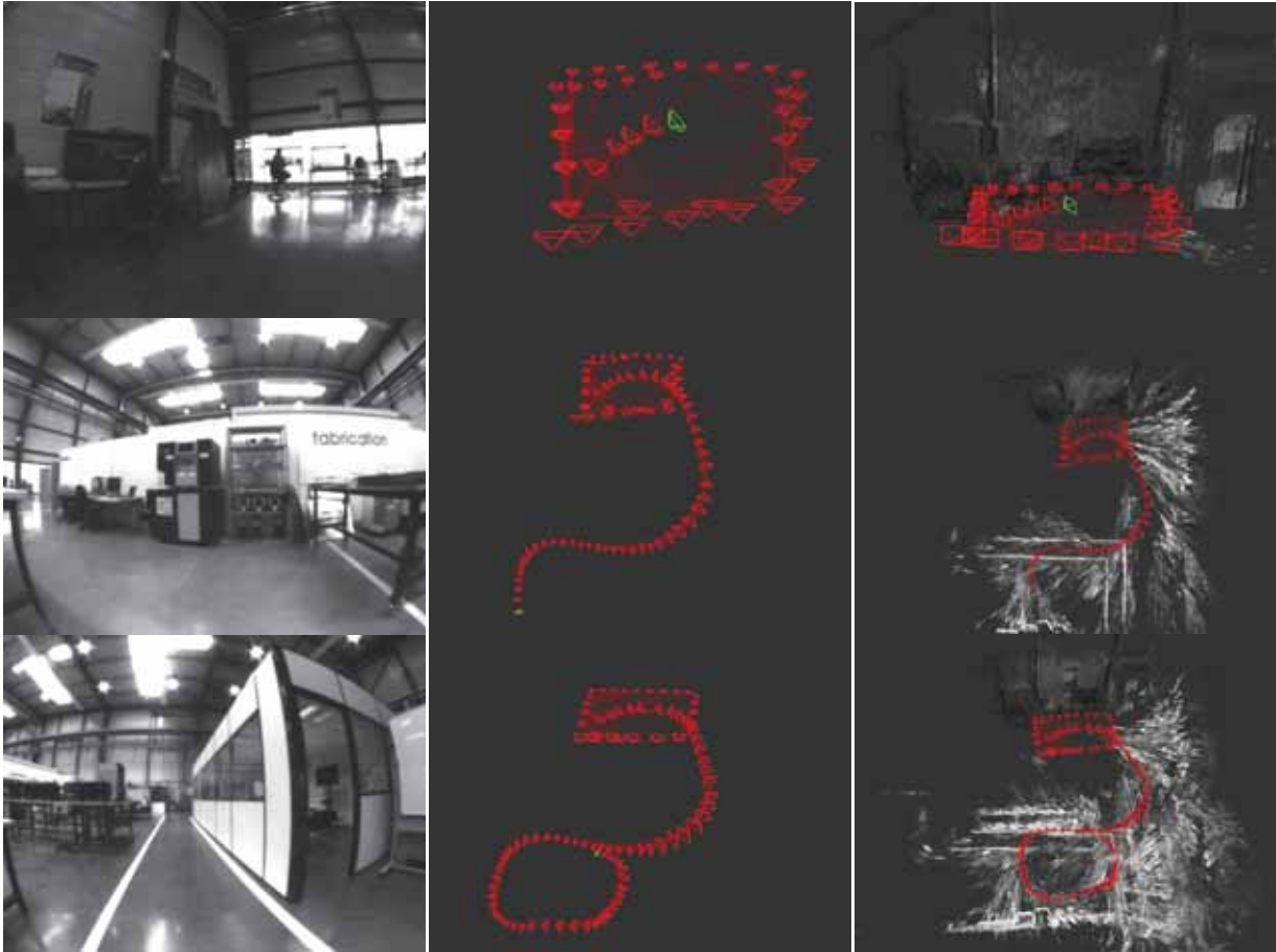
Fig. 3. Monocular SLAM Process on robot R1 at three different instants. Left: Image captured by the camera. Middle: Trajectory built by the robot. Right: Map built by the robot.
