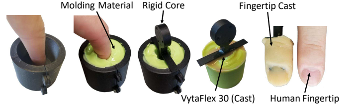
Fig. 6. The process of creating a cast of a human fingertip. We first make a mold out of Kulzer's Flexitime Correct Flow; then we insert a rigid core and fill the void with Smooth-On VytaFlex 30 to make the fingertip cast. The rigid core is later attached to a Nano17, as in Fig. 3b, creating a sensor that outputs a six-element vector of the forces and torques acting on the fingertip.
