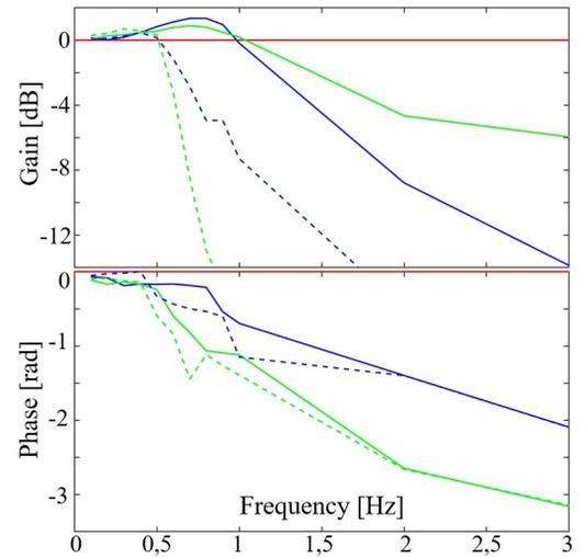
Fig. 4. Bode plots obtained for the sinusoidal responses for the pan axis (blue) and tilt axis (green). The dotted lines show the frequency response in the worst-case scenario (amplitude  $A = 90^\circ$ ) while the full lines show the frequency response for a mean scenario (amplitude  $A = 45^\circ$ ).
