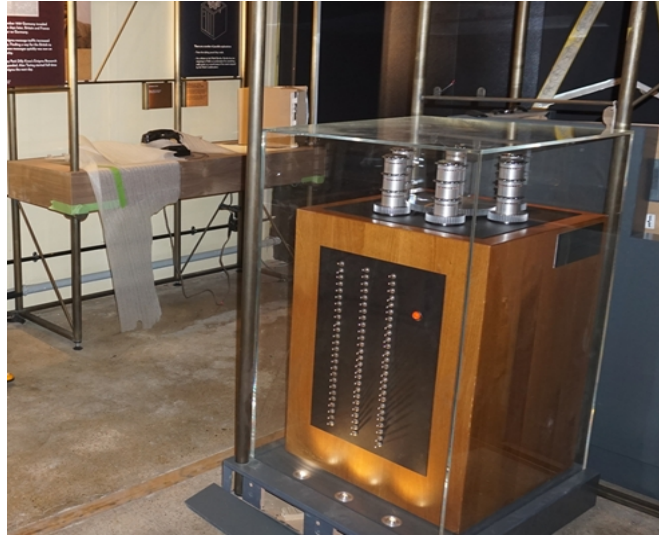
Fig. 12. Reconstruction of Rejewski's "bomba" at Hut11A, Bletchley Park
