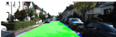
Fig. 7. Visual representation of the results. The generated image was provided by KITTI Evaluation Server. Green pixels represents true positives, red pixels are false negatives and blue pixels are false positives.
