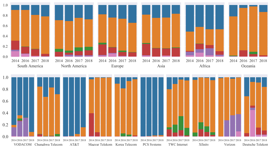
Fig. 4. NAT type distribution by continent in 4 different years (top) and NAT type distribution by the top 10 providers in 4 different years (bottom). Colors represent types as defined in Figure 3.
