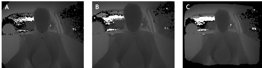
Fig. 3 Data augmentation strategy. (A) Original depth image; (B) Augmented image that simulates the positioning of the camera closer to the driver; (C) Augmented image that simulates the camera being located farther from the driver
