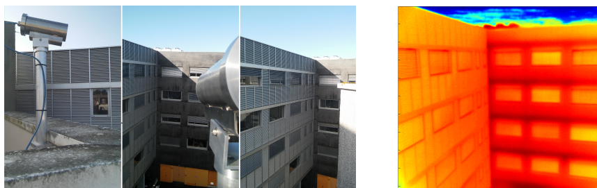
Figure 15: Inria test bed, and main IR image around sunrise.
