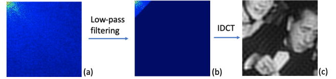
Figure 2. Coefficients selection (a) Coefficients \mathbf{F}(u, v) after the DCT (see Fig 1) (b) Low-pass filtering. Selection of the coefficients using the zig-zag algorithm (c) Image reconstruction using the IDCT.
