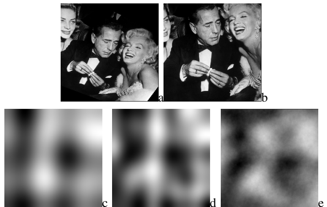
Figure 6. Simulated experiment: (a) initial image, (b) desired image, IDCT of the initial image for (c) K = 20 (d) K = 50 , (e) reconstructed image with the PCA with K = 50
