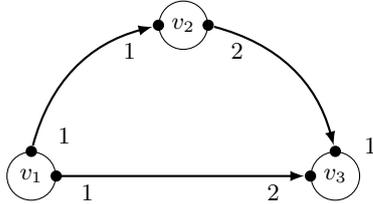
Figure 3: A simple *synchronous dataflow* graph with three nodes  $v_1, v_2$  and  $v_3$  with only one input port and one output port for each of them. Data flows from  $v_1$  to  $v_3$ , from  $v_1$  to  $v_2$  and from  $v_2$  to  $v_3$ .  $v_1$  yields 1 token per firing, and  $v_3$  requires 2 tokens to be fired.  $v_1$  is a *source* node,  $v_3$  a *sink* node.
