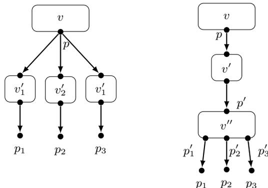
Figure 6: Node  $v$  has one output port,  $p$ , which is connected to three input ports,  $p_1, p_2, p_3$ . On the left, we insert a resampler on each edge  $p \rightarrow p_1, p \rightarrow p_2, p \rightarrow p_3$  whereas on the right, we insert a node  $v''$  with one input port  $p'$  and 3 outputs  $p'_1, p'_2, p'_3$ , and we insert the resampler  $v'$  on edge  $p \rightarrow p'$ .
