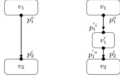
Figure 4: Inserting a downsampling node  $v'_1$  between nodes  $v_1$  and  $v_2$ .  $v_1$  has an output port  $p_1^o$ ,  $v_2$  has an input port  $p_2^i$  and  $v'_1$  has an input port  $p_1'^i$  and an output port  $p_1'^o$ .
