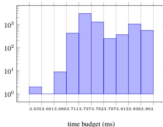
Figure 1: Histogram of relative deadlines for the *audio callback* on a MacBookPro with macOS. We execute a C++ test program generating a sawtooth signal for 10 s. The time budgets range from 3.64 ms to 3.89 ms, *i.e.* a 254  $\mu$ s jitter, with a mean of 3.78 ms
