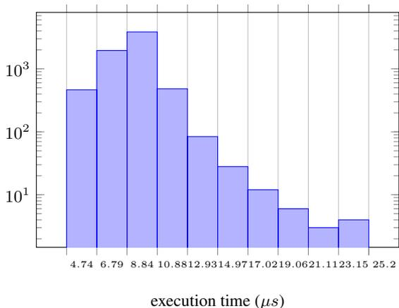
Figure 2: Histogram of the execution time for the same code generating a saw signal for 10s. Here, we show the execution time at each cycle in the *audio callback* for generating a sawtooth signal on a MacBookPro with macOS. The execution times range from 4.74 μs to 25.20 μs with an average of 9.17 μs. The standard deviation is 1.59 μs.
