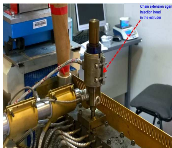
Figure 3. Photo of the used mixing head coupled to the metering pump for the injection of the chain extender agent onto the molten prepolymer in the extruder.
