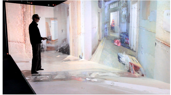
Figure 3: Immersive navigation in the point cloud in a large CAVE-like structure.
