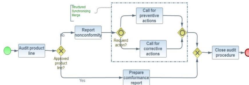
Fig. 3. Structured synchronizing merge in BPMN
