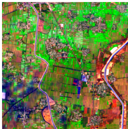
(b) Landsat8 OLI band652 synthetic data and band8 panchromatic image after fusion of local mapimage local map
