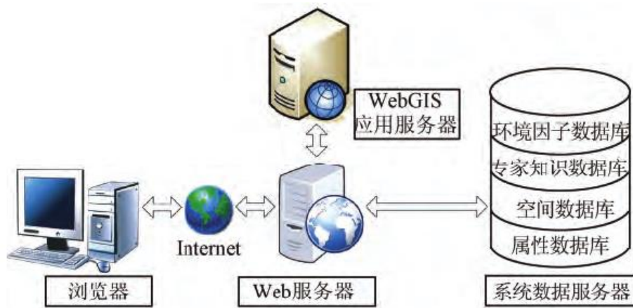
Figure. 1. Structure of agricultural environmental dataanalysis
