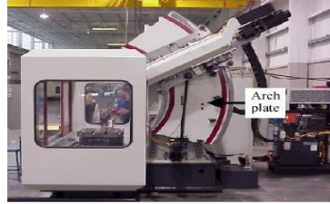
Fig. 1. Reconfigurable machine tool (RMT) developed at the ERC-RMS [4]
