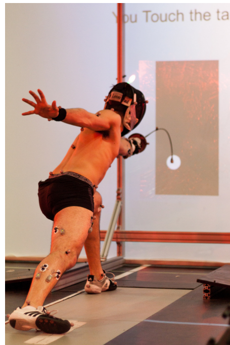
Figure 4. End of a successful lunge trial with a big target (0.10m diameter). Success information was displayed in real time by the system on the top of the plastron. Muscle activity and motion of the fencer were captured for further investigations.
