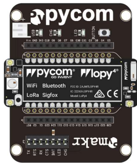
Fig. 6. Pycom module composed of a LoPy4 and an Expansion Board [17].
