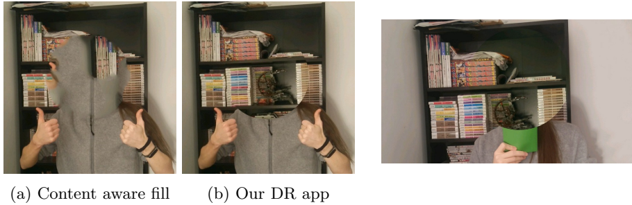
Fig. 7: Comparison of inpainted frames using Adobe Photoshop’s PatchMatch-based content-aware fill and output of our DR application.
