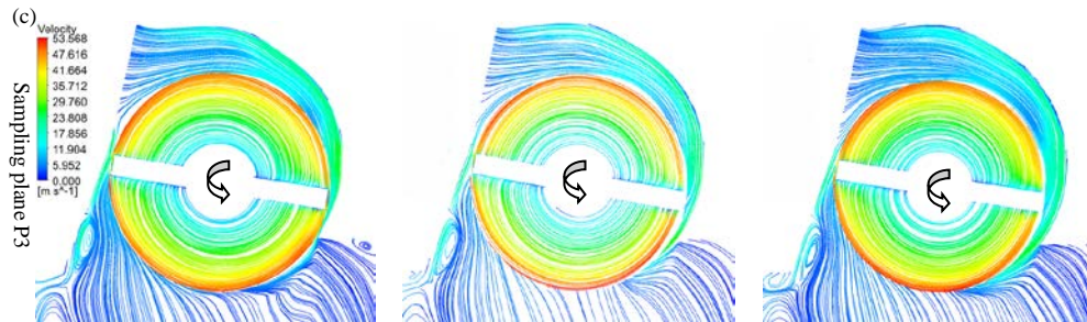
Fig. 30. Streamlines on P1, P2 and P3 under different flail tip clearances
