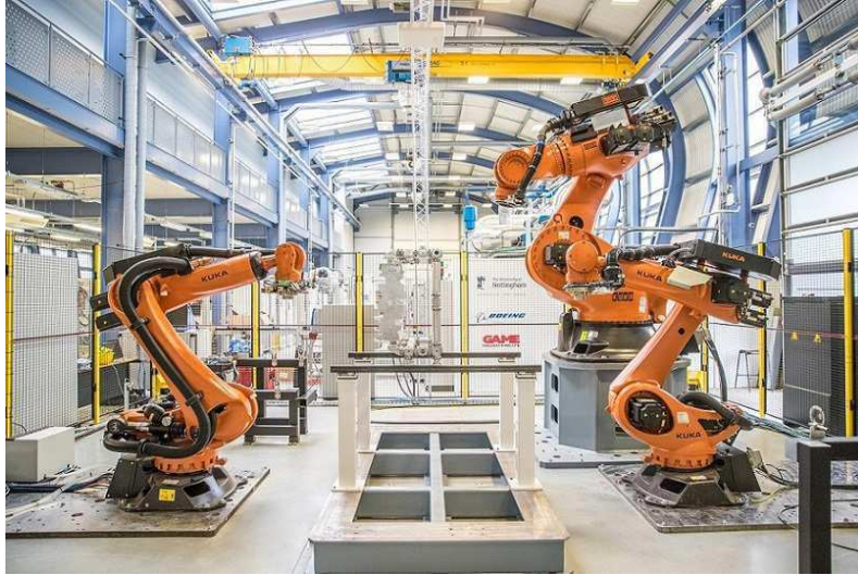
Fig. 3. Reconfigurable assembly cell of the Future Automated Aircraft Assembly Demonstrator developed by the University of Nottingham
