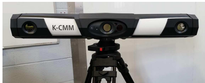
Fig. 5. K-CMM camera of the FA 3 D
