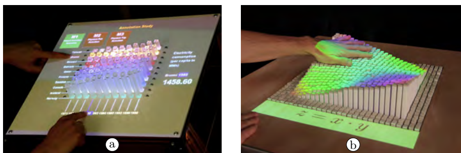
Fig. 21: (a) The EMERGE shape display featuring 10 by 10 bars [152]; (b) The inFORM shape display featuring 30 by 30 bars [41].
