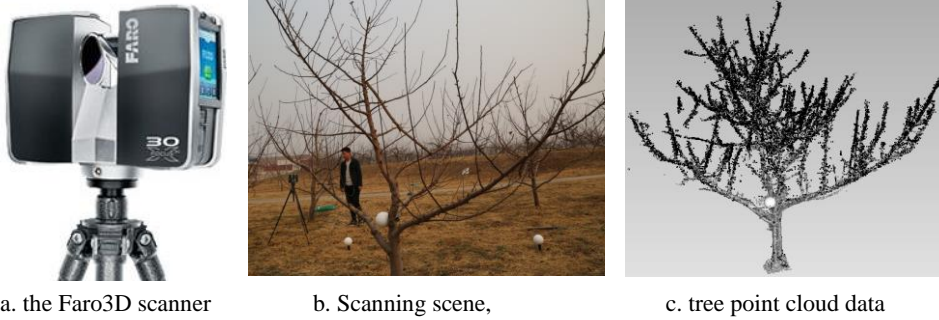
Fig. 4. The equipment and rule diagram of crown digitizer
