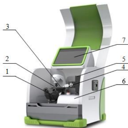
Fig.2. System structure chart: 1. Microscope and CCD imaging module; 2. Detection pond; 3. Ion-selective microelectrode; 4. First signal amplifier; 5. Macro 3D automatically controlled platform; 6. Signal gathering/motion control/data analysis modules; 7. Touchscreen.
