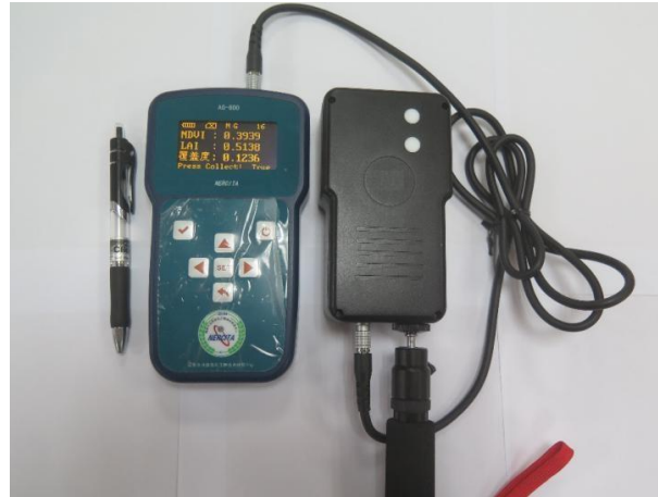
Fig. 3 Instrument for measuring crop growth parameters
