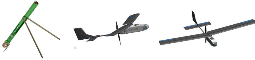
Fig. 2. Concept of launch system and tube deployable small UAV
