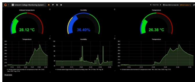
Fig. 7. Main Dashboard with graphical charts and data history for each of the three sensors
