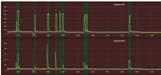
Fig. 12. Colorized areas with occupied (green) and vacant (brown) seat state for CapSense module
