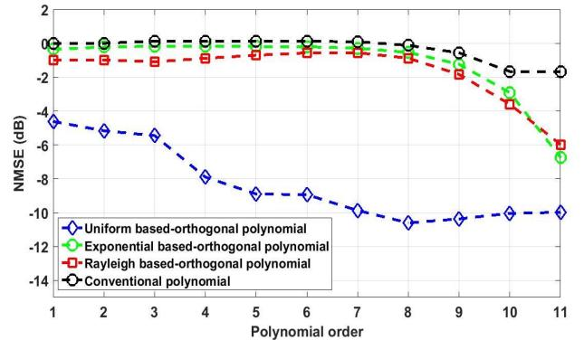
Fig. 4. The HPA modelling error comparison at IBO = 4
