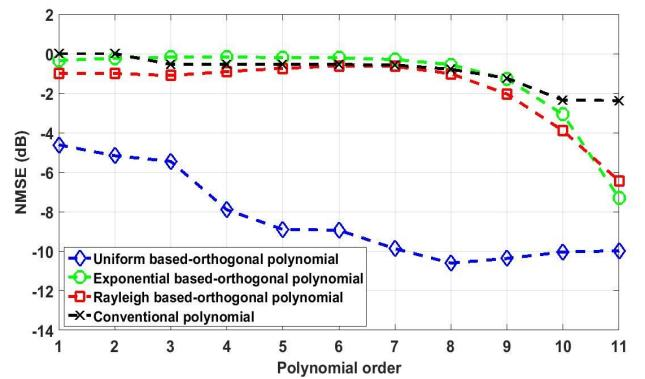
Fig. 5. The HPA modelling error comparison at IBO = 6
