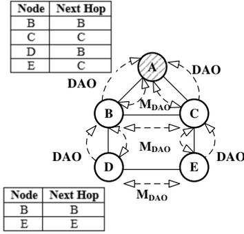
Fig. 2. P2MP and P2P Routing Using Multicast DAO
