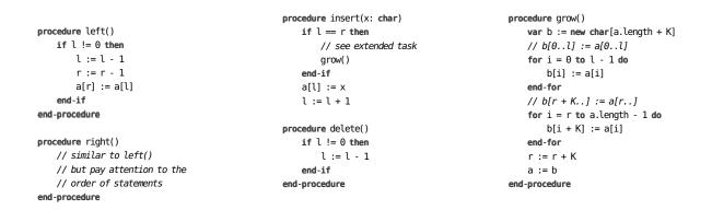
Fig. 1. Gap Buffer implementation in pseudo-code.
