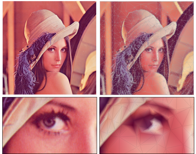
Fig. 15. Image compression by Delaunay point process. A Delaunay triangulation with only 2.8K colored points (right) is sufficient to approximate a 262Kpixels image (left) with a structural similarity (SSIM) greater than 0.97. Each triangle is colored by bilinear interpolation of its three vertices. Here we display the Delaunay edges in grey for visualization.
