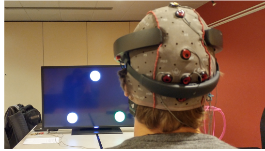
Fig. 1: Experimental setup of Study 1: the user wears an EEG cap as well as the HoloLens. In this particular condition, the SSVEP targets were displayed on the screen.
