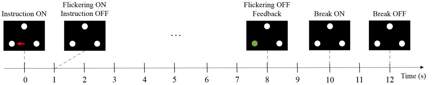
Fig. 2: Trial timing. ( $t=0s$ ) The user is instructed to focus on a particular target through an arrow. ( $t=1s$ ) The arrow disappears and all targets flicker for 7s. ( $t=8s$ ) The flickering stops and a sham feedback is provided (the designated target is highlighted in green in 80% of the trials). ( $t=10s$ ) A two-second break starts before the next trial begins.
