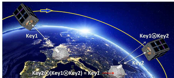
Figure 1 Global unconditionally secure quantum key distribution through a trusted node in uplink configuration [21]
