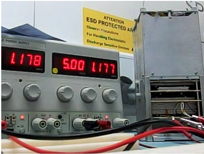
Fig. 9: DS-1: Burnwire Testing.
