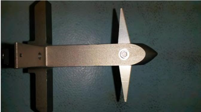
Fig. 14: **Harpoon Barb Mechanism**. This figure shows the projectile with the barbs deployed.
