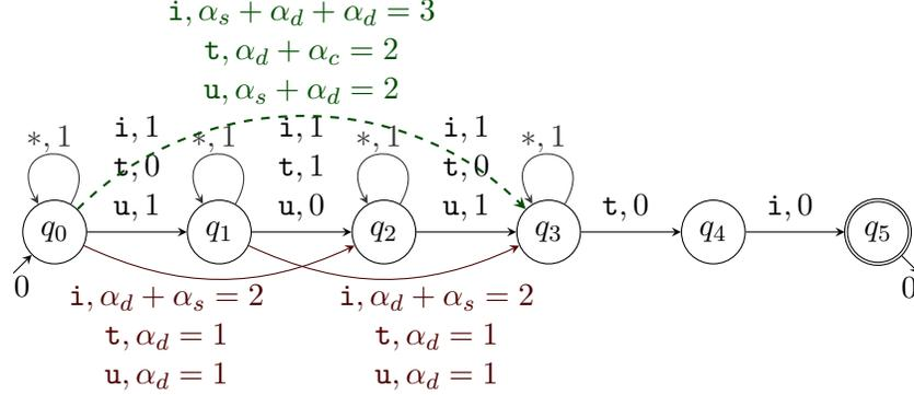
Figure 7: Automaton  $\mathcal{A}_{\text{tutti}}^E$  on the tropical semiring after solving  $w_{i,a,j}$  for every  $a \in \Sigma_3$  and every  $i$  and  $j$  with  $0 \leq i \leq j \leq 3$ , considering the ruleset  $E_0 \cup E_{3,c}$ . All edition rules have here a weight of 1. Solving  $w_{0,t,3}$  is done through the  $x_{0,t,3}$  variable. By equation (3), we have:
