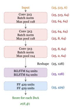
Fig. 2. Architecture of the network.
