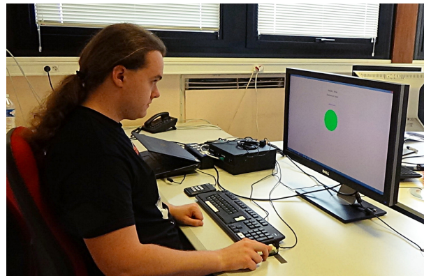
Fig. 5: Experimental setup. A participant perceives a letter using skin stretch at his index, and enters his choice (letter) using the keyboard with his non-dominant hand.
