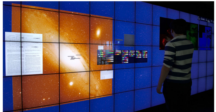
Figure 2. FITS-OW on WILDER showing multiple FITS images, the result-set of a SIMBAD query restricted to observations about galaxies, basic measurements for galaxy M31, a page of a research paper discussing that particular galaxy, and the color map selector.
