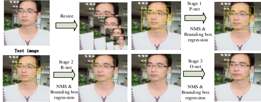
Fig. 2. Joint face detection and alignment using multitask cascaded convolutional networks.
