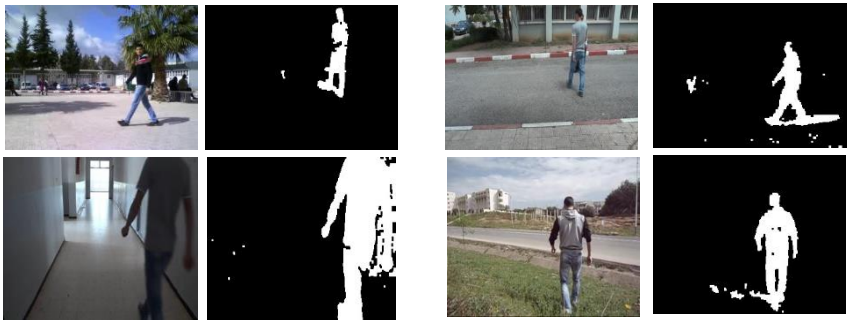
Fig. 2. Background subtraction results in personnel video database in both indoor and outdoor environments
