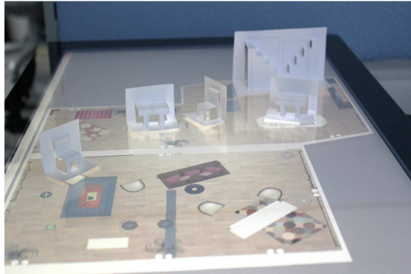
Fig. 1. A room layout design application in which the user can move the interactive pop-up card interface on the table to manipulate the furniture layout in a room.
