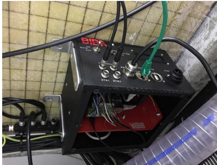
Fig. 2. The Universal Marine Gateway as implemented on final Hydrolift P-42 prototype
