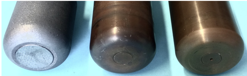
Figure 1: ESA standard probes (5 cm diameter) used for the measurements performed in the Plasmatron facility: (left to right) stagnation-point probe holding a material sample, copper calorimeter, and water-cooled Pitot probe.
