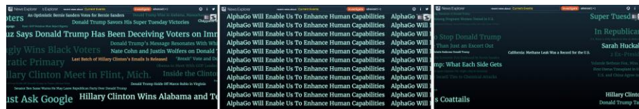
Fig. 5. The Panta Rhei can draw attention to a particular tick using color (top), uniformity (middle), or isolation (bottom).
